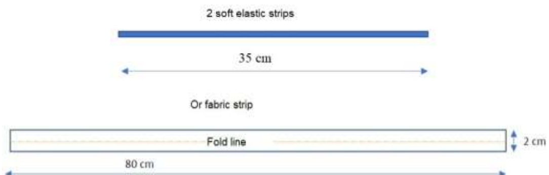
Figure 8 — Flat-fold - Sizing of the head harness
