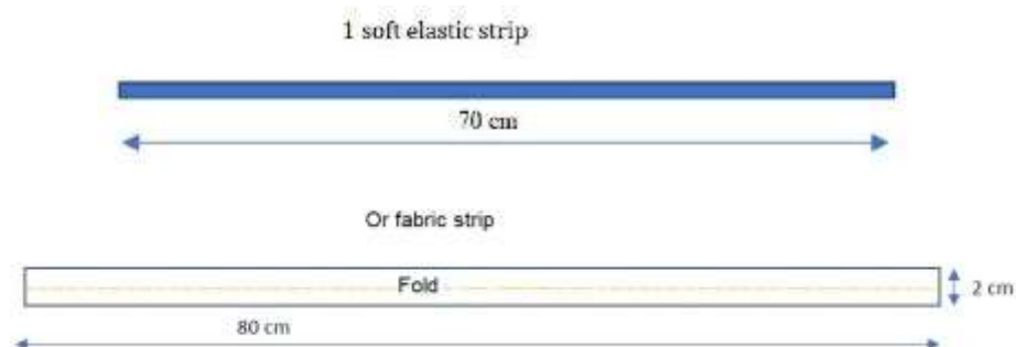
Figure 5 — Duckbill - Sizing of head harness
